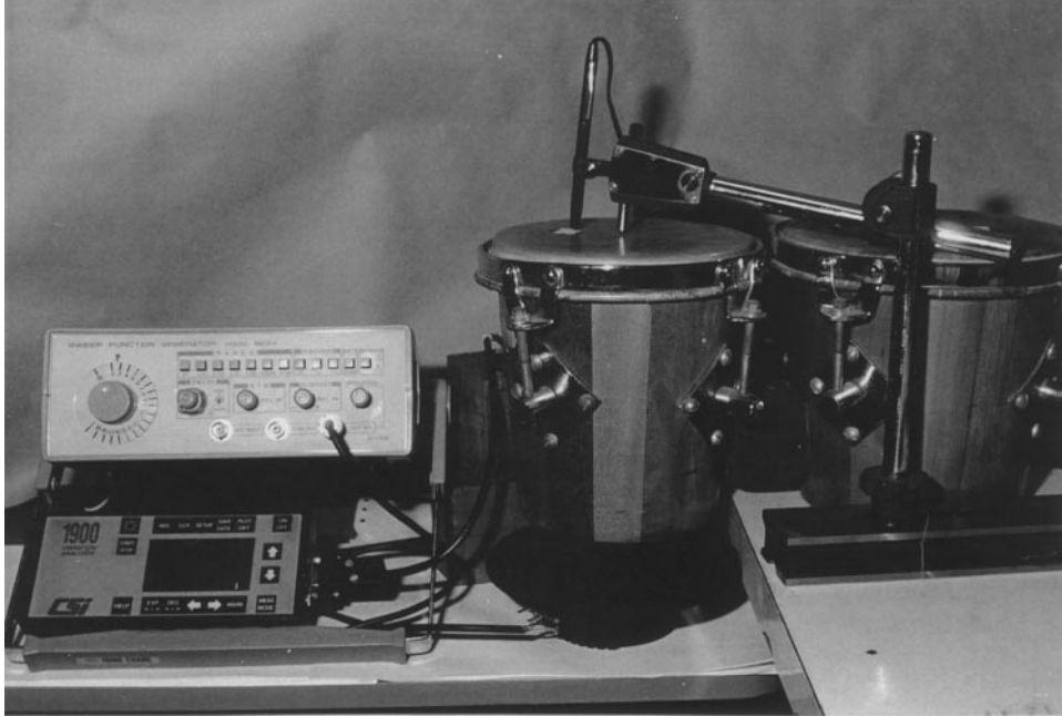
Figure 1. Experimental set-up and test of the circular membrane.
